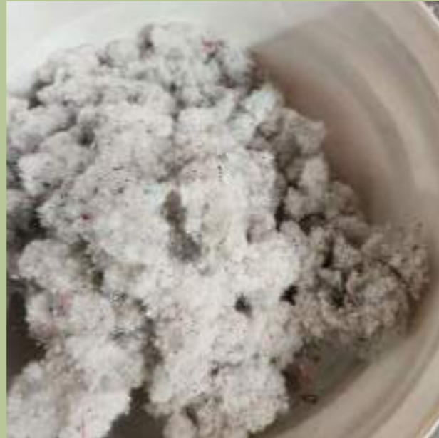
Small amount of residual PVC in Polyester wool after separation, posing the final hurdle in the PVC Separation process.
